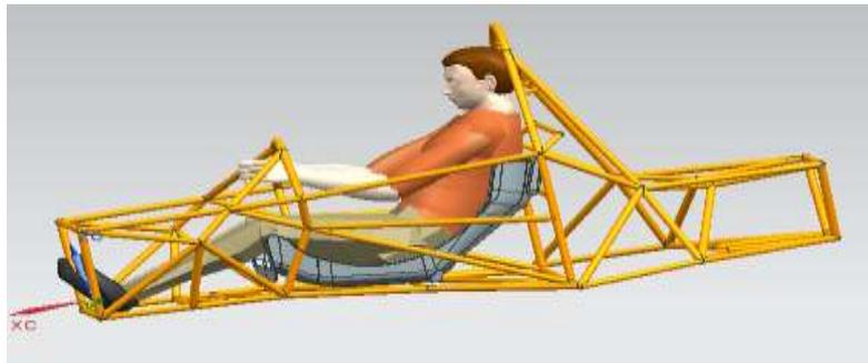
Fig.9 complete assembly drawing
